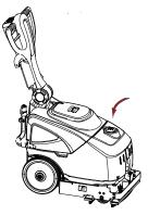
Adjust the slope of the handle by pulling the handle release lever.
