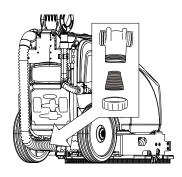
Check the dirty water tank float is undamaged and clean and moves freely on the pin.
