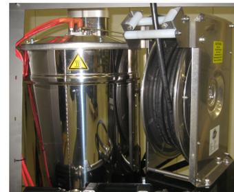
The powerunit is completed built on a frame, together with the fuel tank, installed in a completely covered foolding hood with gas springs, which can be opened/closed.
