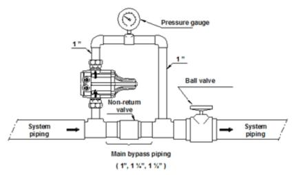
In the event of the pressure losses caused by the installation of the PRESSCONTROL taking the system flow rate down below the desired value, it is possible to install the PRESSCONTROL in bypass as indicated in the figure .
