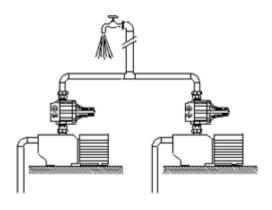
Two PRESSCONTROL devices with different restart pressure calibrations (T 1.2 bar and T 1.5 bar ).
