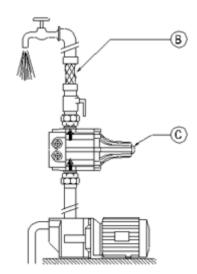
It is recommended to connect the output of the device to the plant by means of a ball valve and flexible tube (fig. B).
