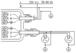
Connection of two pumps with a total input exceeding 1.5 kW (2 HP).
