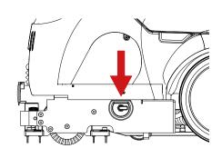
Press the ON-OFF button, then press the brush button to activate suction and water delivery.
