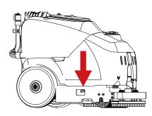
Remove the cap for STANDARD operation from its housing, and replace it with the cap for CARPET KIT operation.
