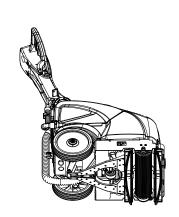
Insert the Carpet Kit carpet cleaner in the front housing, attaching it to the support.
