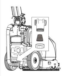
Check the dirty water tank float is undamaged and clean and moves freely on the pin.
